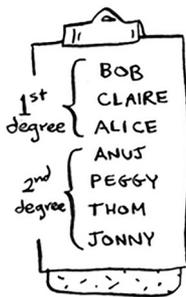
Another way to see this is, first-degree connections are added to the search list before second-degree connections.
