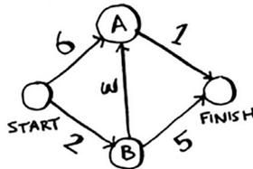
Each segment has a travel time in minutes. You'll use Dijkstra's algorithm to go from start to finish in the shortest possible time.
