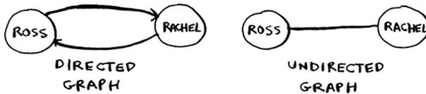
An undirected graph means that both nodes point to each other. That's a cycle!
