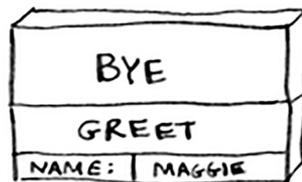
A box for that function is added to the top of the stack. Then you print `ok bye!` and return from the function call.
