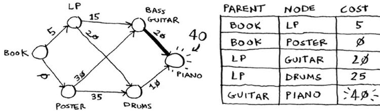
Ok, you finally have a price for the piano, by trading the guitar for the piano. So you set the guitar as the parent. Finally, the last node, the drum set.
