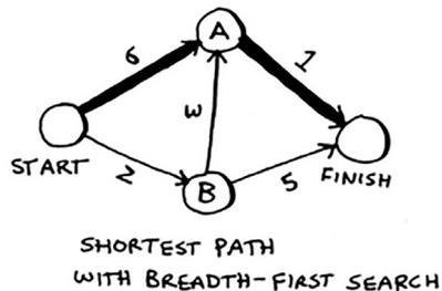
In the last chapter, you used breadth-first search to find the shortest path between two points. Back then, “shortest path” meant the path with the fewest segments. But in Dijkstra’s algorithm, you assign a number or weight to each segment. Then Dijkstra’s algorithm finds the path with the smallest total weight.
