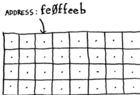
fe0ffeeb is the address of a slot in memory.
