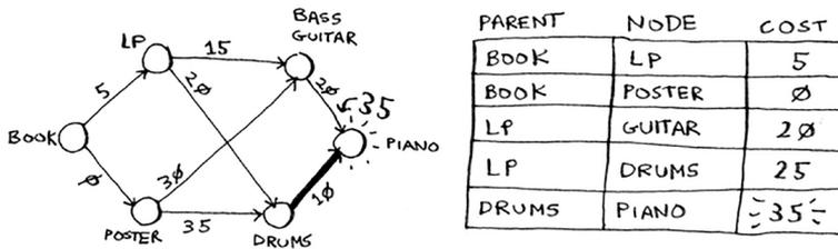
Rama can get the piano even cheaper by trading the drum set for the piano instead. So the cheapest set of trades will cost Rama \$35.
