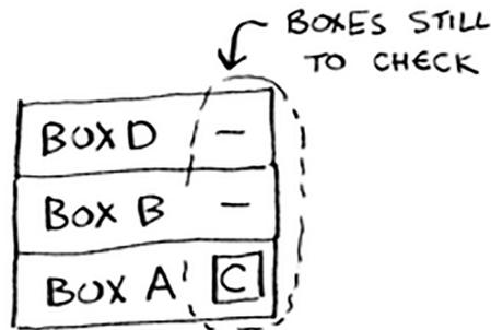
The “pile of boxes” is saved on the stack! This is a stack of half-completed function calls, each with its own half-complete list of boxes to look through. Using the stack is convenient because you don’t have to keep track of a pile of boxes yourself—the stack does it for you.
