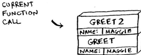
Your computer is using a stack for these boxes. The second box is added on top of the first one. You print `how are you, maggie?` Then you return from the function call. When this happens, the box on top of the stack gets popped off.
