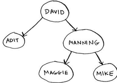
For every node, the nodes to its left are *smaller* in value, and the nodes to the right are *larger* in value.
