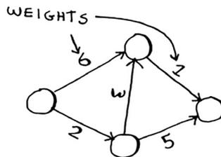
A graph with weights is called a *weighted graph*. A graph without weights is called an *unweighted graph*.
