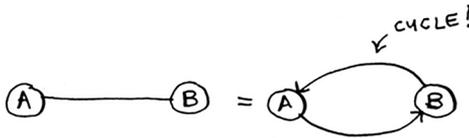
With an undirected graph, each edge adds another cycle. Dijkstra's algorithm only works with *directed acyclic graphs*, called DAGs for short.
