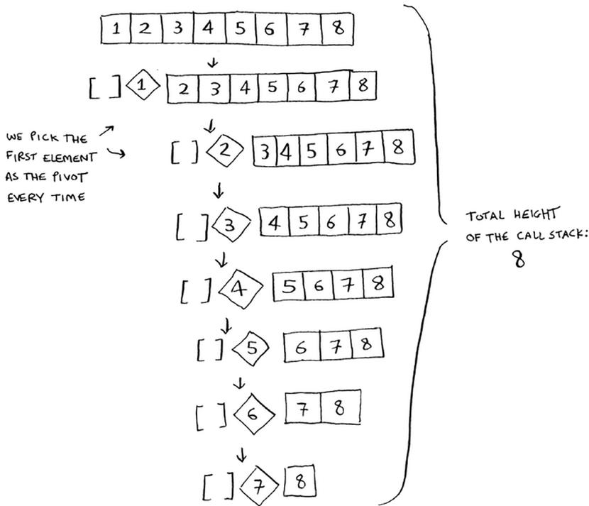
Notice how you're not splitting the array into two halves. Instead, one of the sub-arrays is always empty. So the call stack is really long. Now instead, suppose you always picked the middle element as the pivot. Look at the call stack now.
