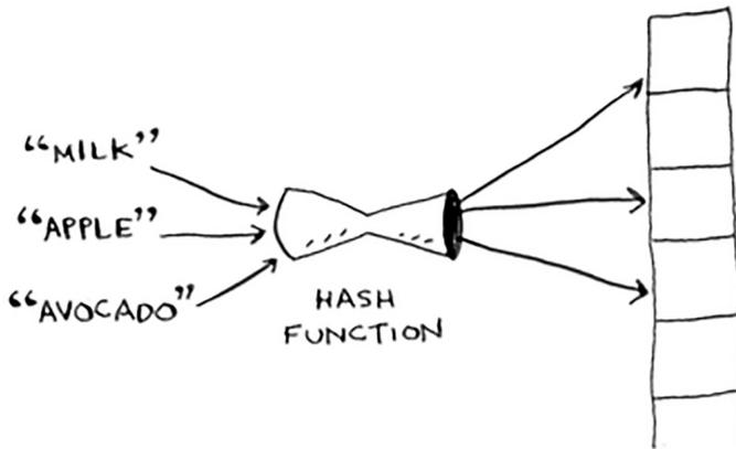
In reality, it's almost impossible to write a hash function that does this. Let's take a simple example. Suppose your array contains 26 slots.
