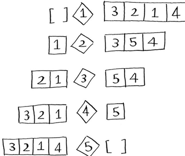
Notice that all of these sub-arrays have somewhere between 0 and 4 elements. And you already know how to sort an array of 0 to 4 elements using quicksort! So no matter what pivot you pick, you can call quicksort recursively on the two sub-arrays.
