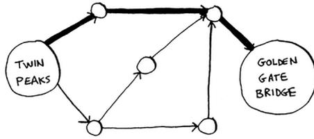
It's not necessarily the fastest path. It's the shortest path, because it has the least number of segments (three segments). But suppose you add travel times to those segments. Now you see that there's a faster path.
