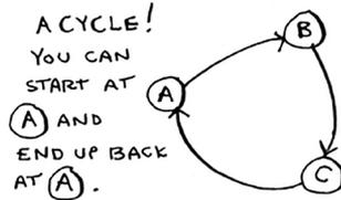
It means you can start at a node, travel around, and end up at the same node. Suppose you're trying to find the shortest path in this graph that has a cycle.
