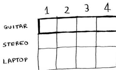
This is the *guitar* row, which means you're trying to fit the guitar into the knapsack. At each cell, there's a simple decision: do you steal the guitar or not? Remember, you're trying to find the set of items to steal that will give you the most value.
