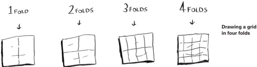
You can “draw” twice as many boxes with every fold, so you can draw 16 boxes in 4 steps. What’s the running time for this algorithm? Come up with running times for both algorithms before moving on.
