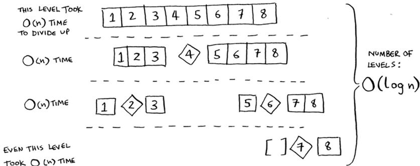
In this example, there are  $O(\log n)$  levels (the technical way to say that is, “The height of the call stack is  $O(\log n)$ ”). And each level takes  $O(n)$  time. The entire algorithm will take  $O(n) * O(\log n) = O(n \log n)$  time. This is the best-case scenario.
