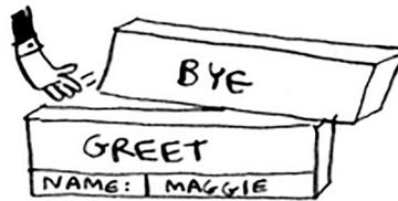
And you're back to the `greet` function. There's nothing else to be done, so you return from the `greet` function too. This stack, used to save the variables for multiple functions, is called the *call stack*.
