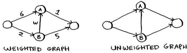
To calculate the shortest path in an unweighted graph, use *breadth-first search*. To calculate the shortest path in a weighted graph, use *Dijkstra's algorithm*. Graphs can also have *cycles*. A cycle looks like this.
