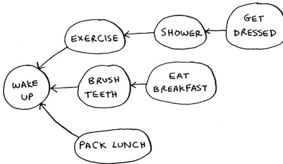
You could say that this list is sorted, in a way. If task A depends on task B, task A shows up later in the list. This is called a *topological sort*, and it’s a way to make an ordered list out of a graph. Suppose you’re planning a wedding and have a large graph full of tasks to do—and you’re not sure where to start. You could *topologically sort* the graph and get a list of tasks to do, in order.
